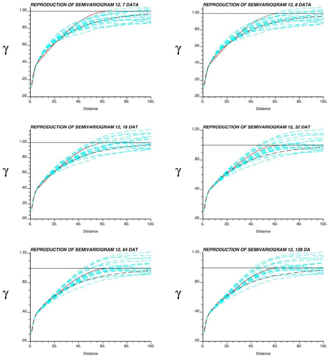
**Figure 5:** Reproduction of the input spherical variogram 12 (see text) by the sequential simulation with increase of the number of data used in simulation. Solid red lines denote the input spherical variogram. Blue dashed lines denote the respective variograms reproduced by sequential simulation. Black dashed lines denote the exponential variogram reproduced by sequential simulation with limited search strategy.
