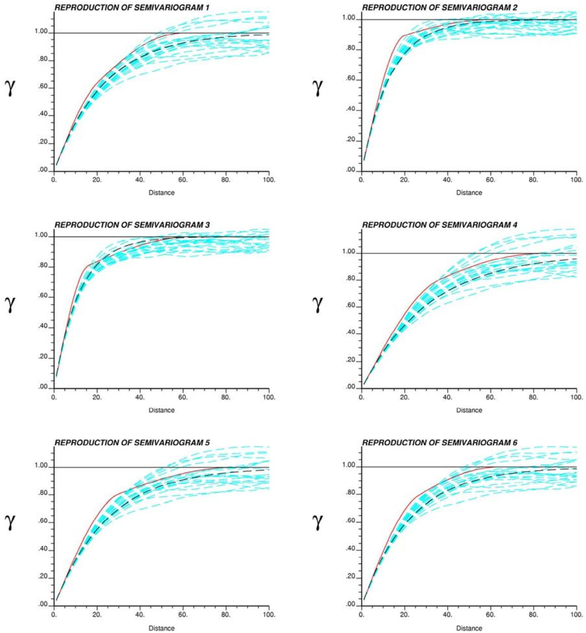
**Figure 2:** Reproduction of the input spherical variogram by the sequential simulation with limited search strategy for the six cases considered in small examples section. Solid red lines denote the input spherical variograms. Blue dashed lines denote the respective variograms reproduced by sequential simulation with limited search strategy. Black dashed lines denote the proposed exponential variograms. (1/2)
