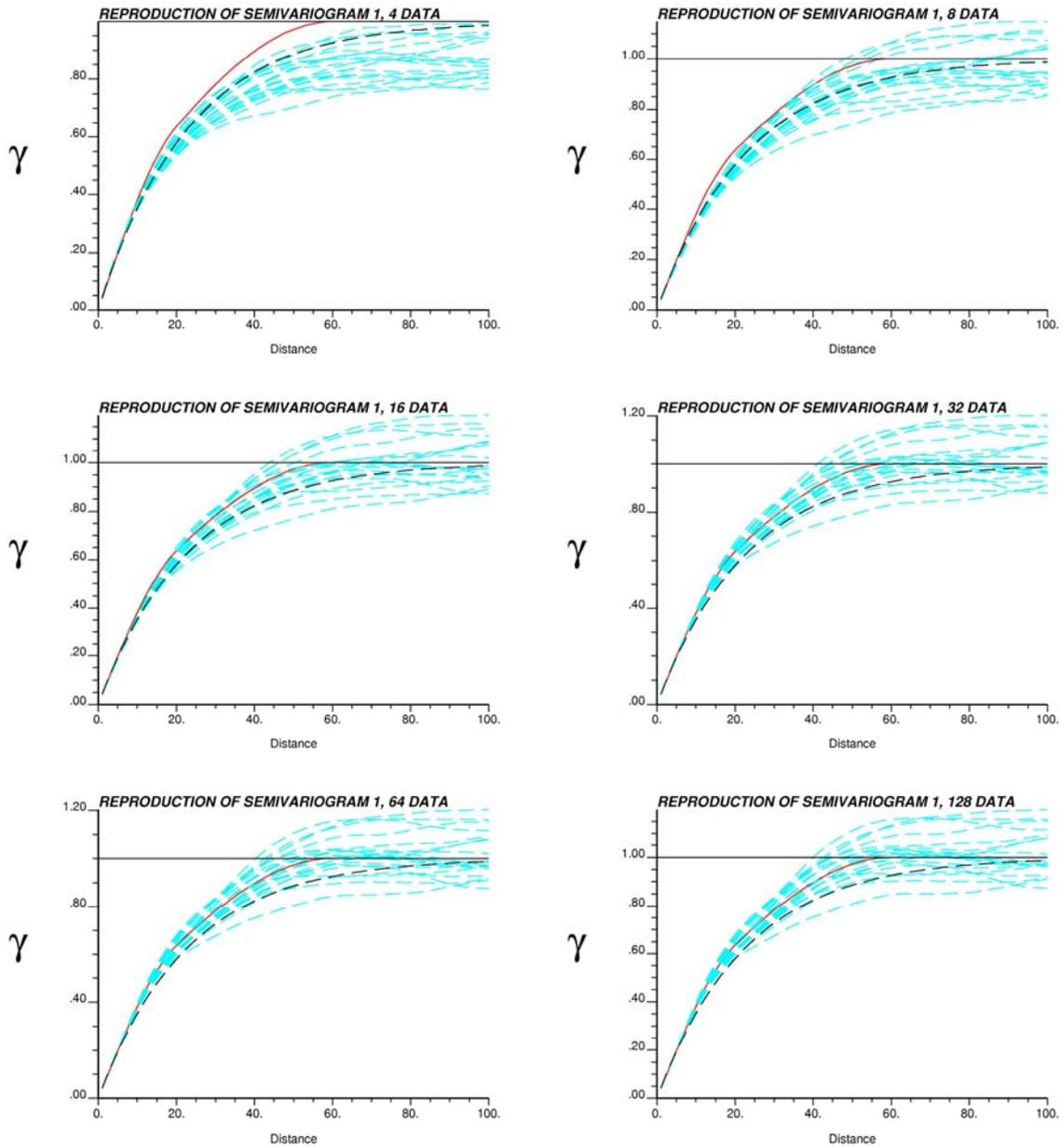
**Figure 4:** Reproduction of the input spherical variogram 1 (see text) by the sequential simulation with increase of the number of data used in simulation. Solid red lines denote the input spherical variogram. Blue dashed lines denote the respective variograms reproduced by sequential simulation. Black dashed lines denote the exponential variogram reproduced by sequential simulation with limited search strategy.
