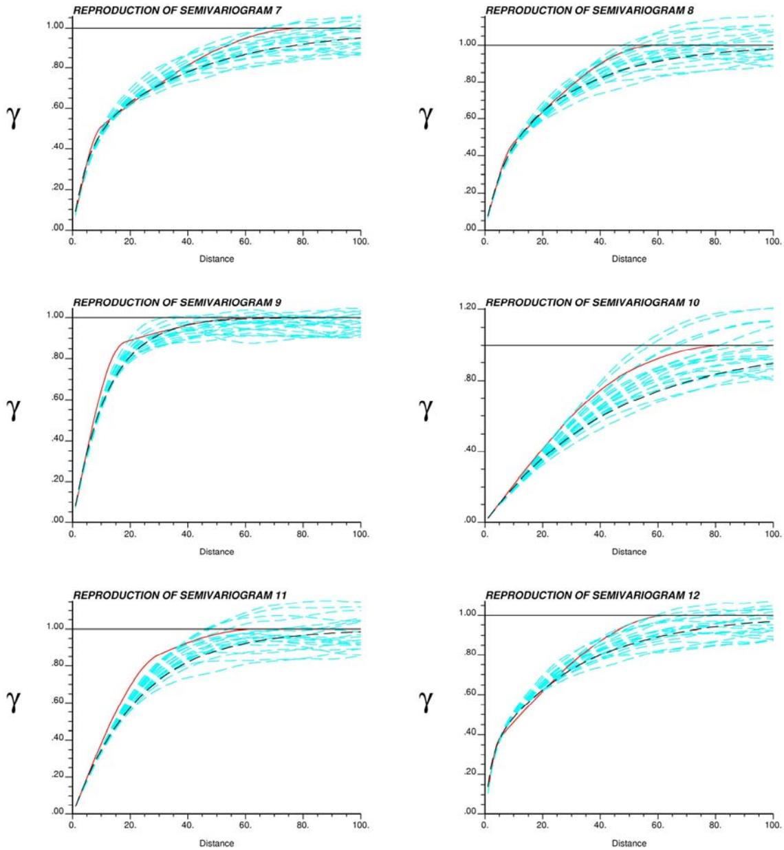
**Figure 3:** Reproduction of the input spherical variogram by the sequential simulation with limited search strategy for the six cases considered in small examples section. Solid red lines denote the input spherical variograms. Blue dashed lines denote the respective variograms reproduced by sequential simulation with limited search strategy. Black dashed lines denote the proposed exponential variograms. (2/2)
