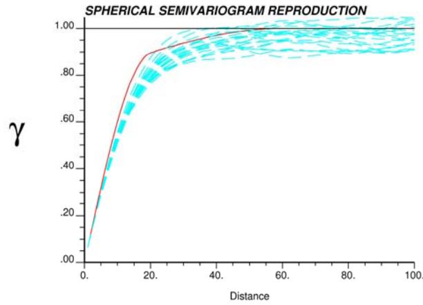
**Figure 1:** Commonly observed problem in reproduction of the input spherical variogram to sequential simulation with limited search strategy. Solid red line denotes the input spherical variogram to sequential simulation. Blue dashed lines denote the variograms reproduced by sequential simulation with limited search strategy.
